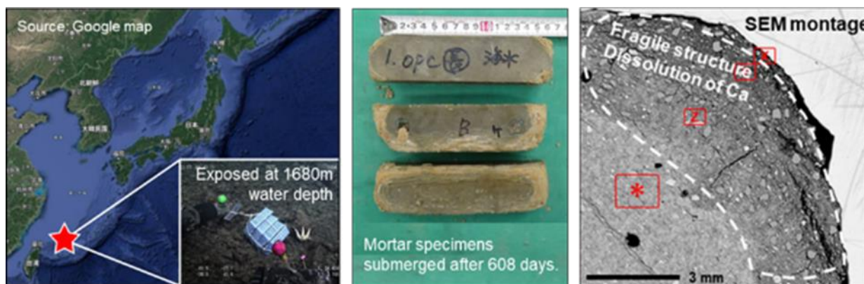
Fig. 2 Map of locations where exposure tests were conducted (left) , mortar specimens exposed in deep-sea for 608 days (middle) (4) , and SEM montage image of cross-section from the specimen (right) .
