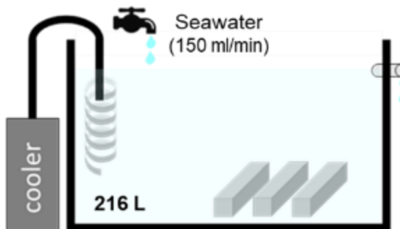
Fig. 3 Experimental set-up of seawater circulation chamber. Fresh seawater was always supplied to each tank at a flow rate of 150 ml/min.
